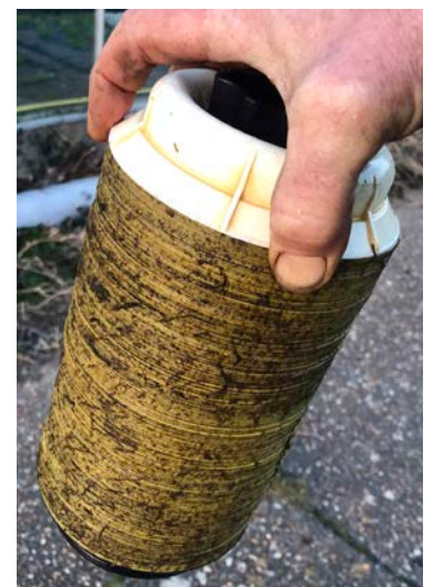
Disc filter overdue for a clean
