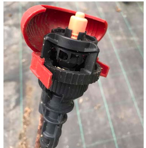
Field sprinkler unit with rod deflector (180 degree spray)
